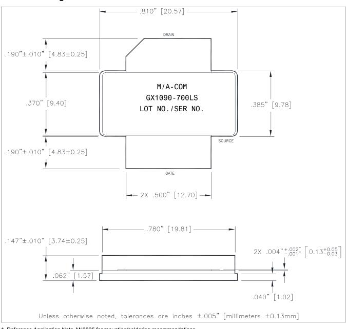
† Reference Application Note AN3025 for mounting/soldering recommendations. Meets JEDEC moisture sensitivity level 1 requirements. Plating is Ni/Au. MACOM
