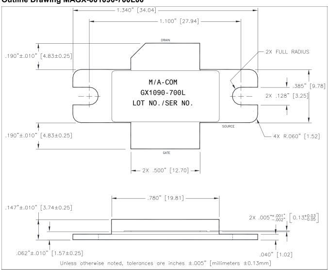
† Reference Application Note AN3025 for mounting/soldering recommendations. Meets JEDEC moisture sensitivity level 1 requirements. Plating is Ni/Au.
