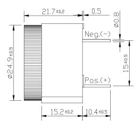
The tolerance for terminal alignment will be  $\pm 1.0 \text{mm}$
