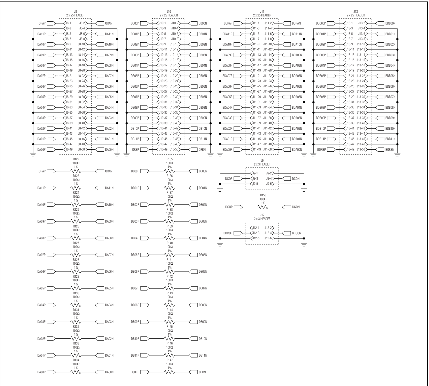
Figure 1e. MAX1217/MAX1218/MAX1219 EV Kit Schematic (Sheet 3 of 7)
