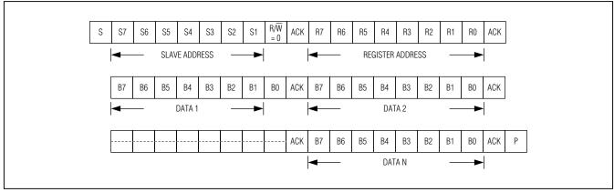
Figure 6. A Burst Write Operation
