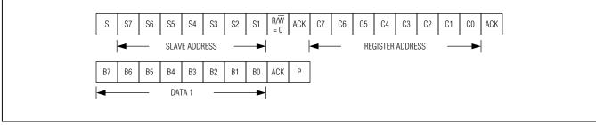
Figure 5. A Single-Byte Write Operation
