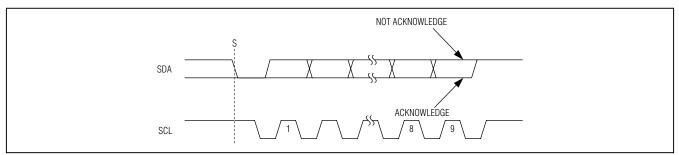
Figure 4. Acknowledge and Not-Acknowledge Bits
