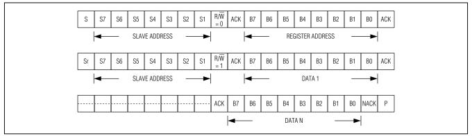
Figure 8. A Burst Read Operation
