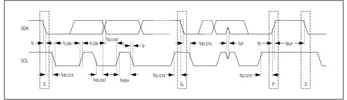
Figure 1. I<sup>2</sup>C Timing
