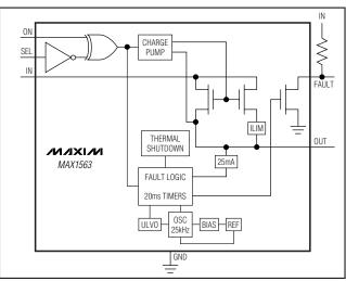
the MAX1562/MAX1562H and 1.35W for the MAX1563, the devices' die temperature exceeds the +160°C thermal-shutdown threshold, and the switch output shuts down until the junction temperature cools by 15°C. The duty cycle and period are strong functions of the ambient temperature and the PC board layout.
