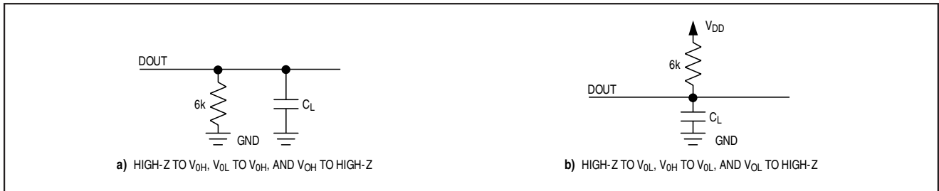
Figure 1. Load Circuits for Enable and Disable Time
