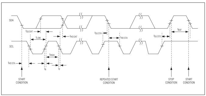
Figure 1. SMBus Timing Diagram
