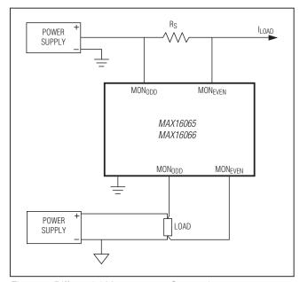
Figure 4. Differential Measurement Connections
