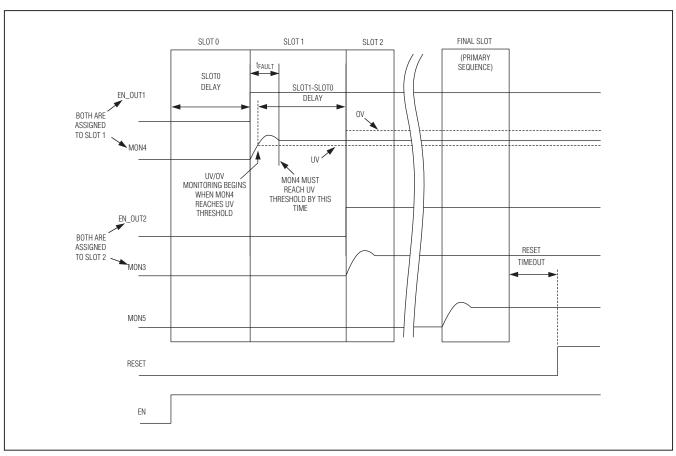
Figure 3. Delay and Reset Timing
