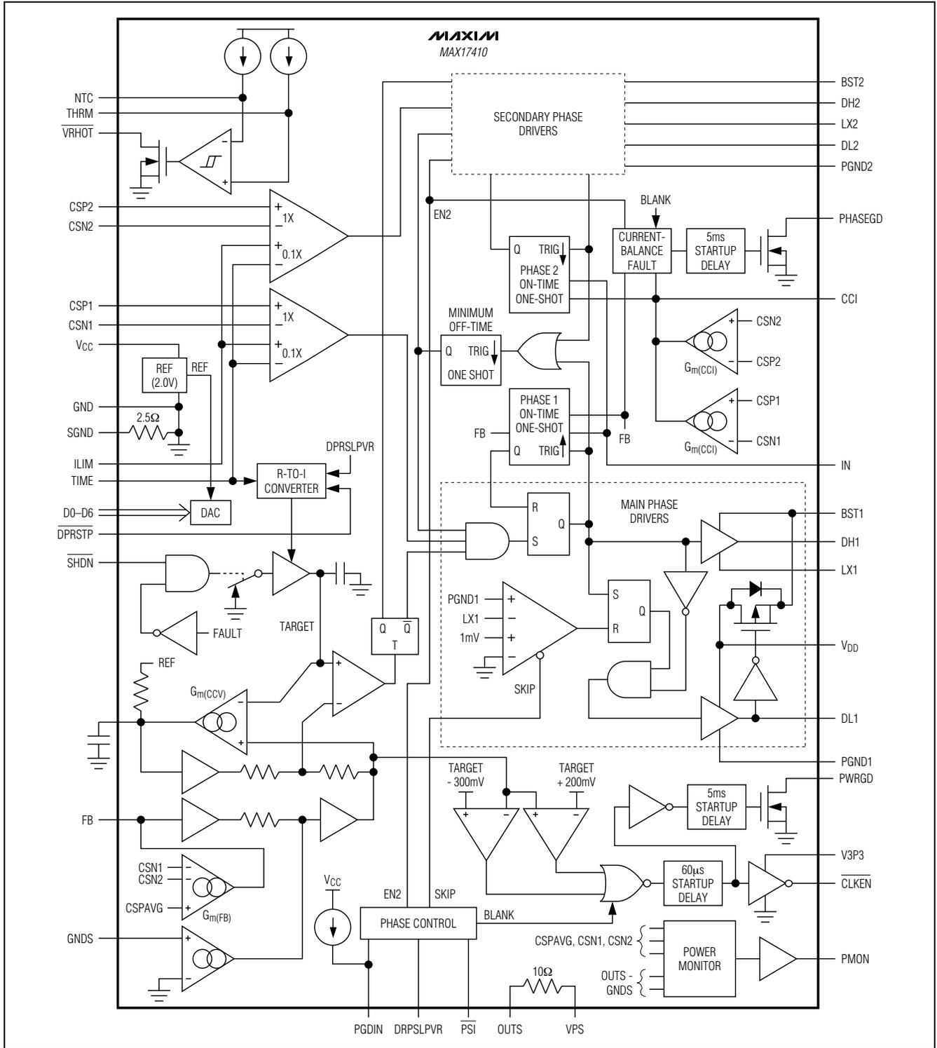
Figure 2. Functional Diagram
