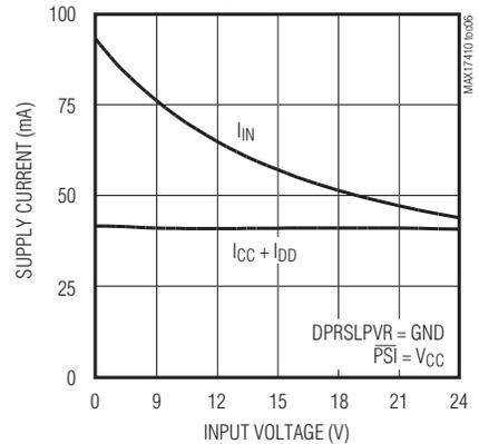
**NO-LOAD SUPPLY CURRENT vs. INPUT VOLTAGE AT SKIP MODE**
