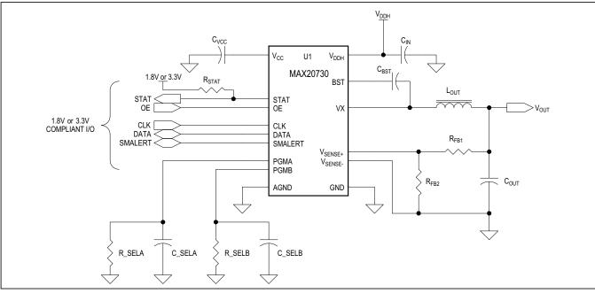
Figure 3. Typical Application Circuit
