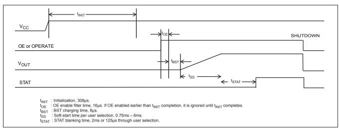
Figure 1. Startup Timing
