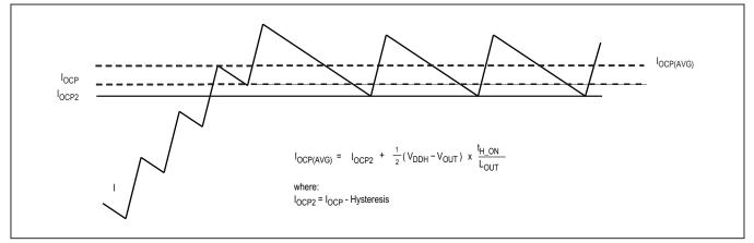
Figure 2. Inductor Current During Current Limiting
