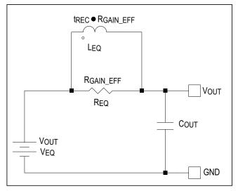
Figure 4. Averaged Small-Signal Equivalent Circuit of Regulator
