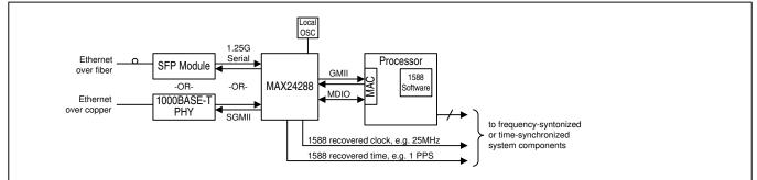
Example 2: Multiport System with Switch-Connected 1588 Slave Node
