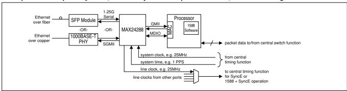
Example 4: Multiport System, Boundary or Transparent Clock, Central Timing Function
