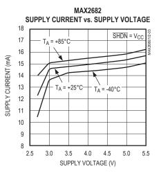
$(\underline{\textit{Typical Operating Circuit}}, V_{CC} = \overline{SHDN} = +3.0V, P_{RFIN} = -25 dBm, P_{LO} = -5 dBm, T_{A} = +25 °C, unless otherwise noted.)$
