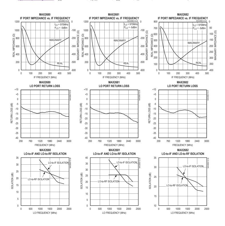
$(\underline{\textit{Typical Operating Circuit}}, V_{CC} = \overline{\text{SHDN}} = +3.0 \text{V}, P_{RFIN} = -25 \text{dBm}, P_{LO} = -5 \text{dBm}, T_{A} = +25 ^{\circ}\text{C}, \text{ unless otherwise noted.})$
