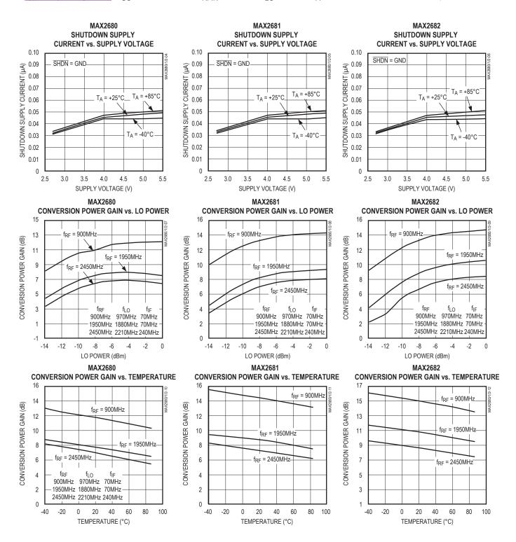
$(\underline{\textit{Typical Operating Circuit}}, V_{CC} = \overline{SHDN} = +3.0V, P_{RFIN} = -25 dBm, P_{LO} = -5 dBm, T_{A} = +25 °C, unless otherwise noted.)$
