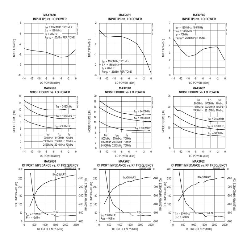
(Typical Operating Circuit, V<sub>CC</sub> = SHDN = +3.0V, P<sub>RFIN</sub> = -25dBm, P<sub>LO</sub> = -5dBm, T<sub>A</sub> = +25°C, unless otherwise noted.)
