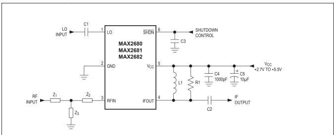
THE VALUES OF MATCHING COMPONENTS C2, L1, R1, Z1, Z2, AND Z3 DEPEND ON THE IF AND RF FREQUENCY AND DOWNCONVERTER. SEE TABLES 2 AND 4.
