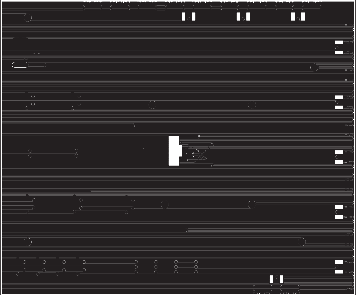
Figure 6. MAX3612 EV Kit PCB Layout—Power Plane
