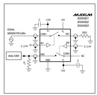
Figure 5. Crosstalk Test Circuit
