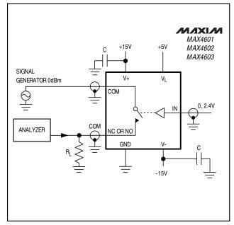
Figure 4. Off-Isolation Test Circuit
