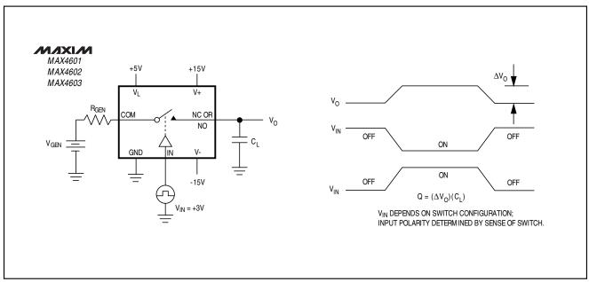
Figure 3. Charge-Injection Test Circuit
