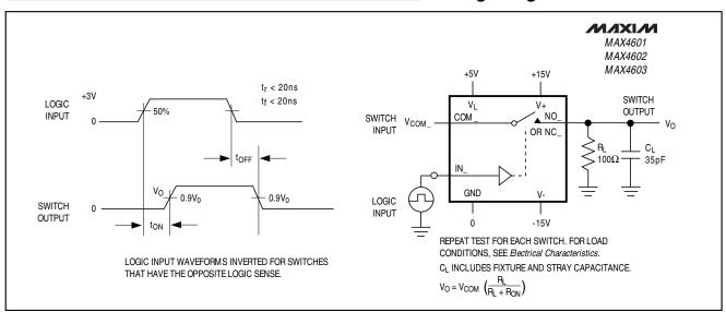
Figure 2. Switching-Time Test Circuit
