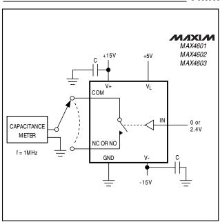
Figure 6. Switch Off-Capacitance Test Circuit
