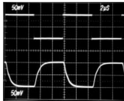
$V_{CC} = +5\text{V}$ ,  $A_v = -1$ ,  $R_L = 10\text{k}\Omega$
