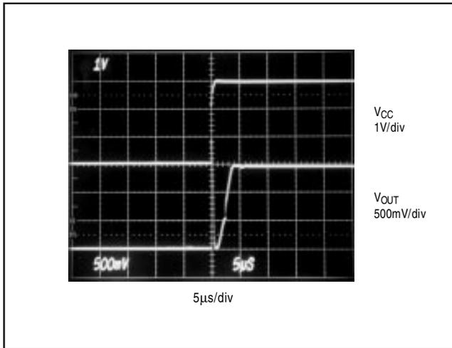
Figure 11a. Power-Up Settling Time ( $V_{CC} = +3V$ )
