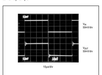
Figure 6. MAX492 Voltage Follower with 1000pF Load ( $R_L = \infty$ )
