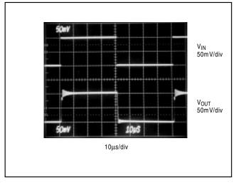
Figure 7b. MAX492 Voltage Follower with 500pF Load— $R_{\rm I}=20{\rm k}\Omega$
