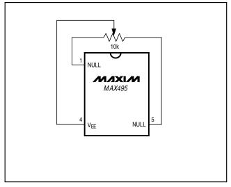
Figure 2. Offset Null Circuit
