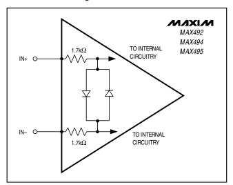
Figure 4. Input Stage Protection Circuitry
