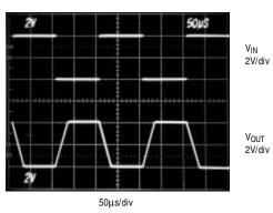
$V_{CC} = +5V$ ,  $A_V = -1$ ,  $R_L = 10k\Omega$
