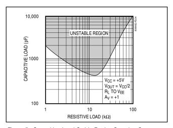
Figure 5. Capacitive-Load Stable Region Sourcing Current
