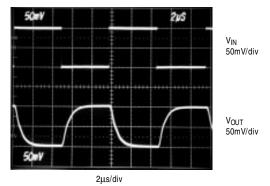
$V_{CC}$  = +5V,  $A_V$  = -1,  $R_L$  = 10k $\Omega$
