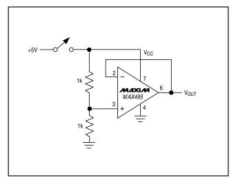
Figure 10. Power-Up Test Configuration
