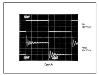
Figure 9a. Driving a 10,000pF Capacitive Load
