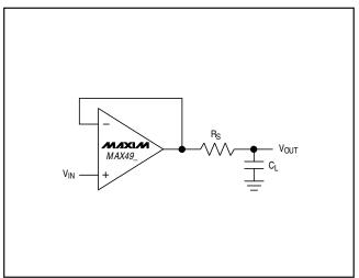
Figure 8. Capacitive-Load Driving Circuit
