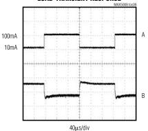
A: LOAD CURRENT B: OUTPUT VOLTAGE: AC-COUPLED, 100mV/div
