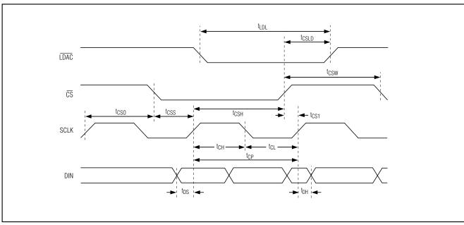
Figure 2. Detailed Serial Interface Timing
