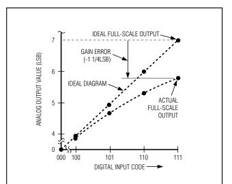
Figure 6d. Gain Error
