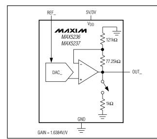
Figure 7. Unipolar Output Circuit (Rail-to-Rail)
