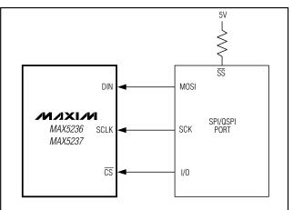
Figure 4. SPI/QSPI Interface Connections
