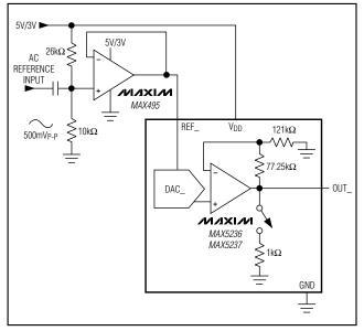
Figure 9. External Reference with AC Components
