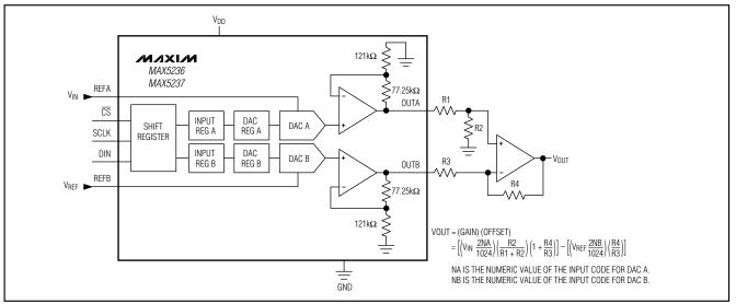
Figure 11. Digital Control of Gain and Offset
