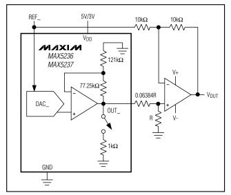
Figure 8. Bipolar Output Circuit
