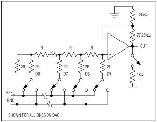
Figure 3. Simplified DAC Circuit Diagram
