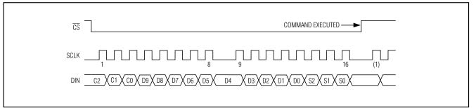
Figure 1. Serial Interface Timing
