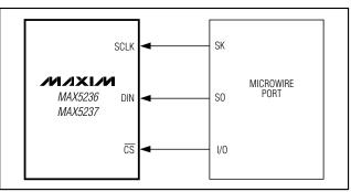
Figure 5. Connections for MICROWIRE
