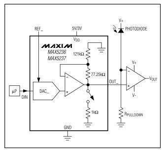
Figure 10. Digital Calibration
