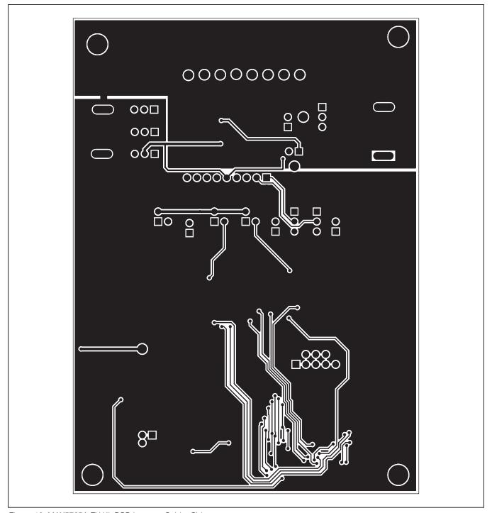
Figure 10. MAX5725A EV Kit PCB Layout—Solder Side
