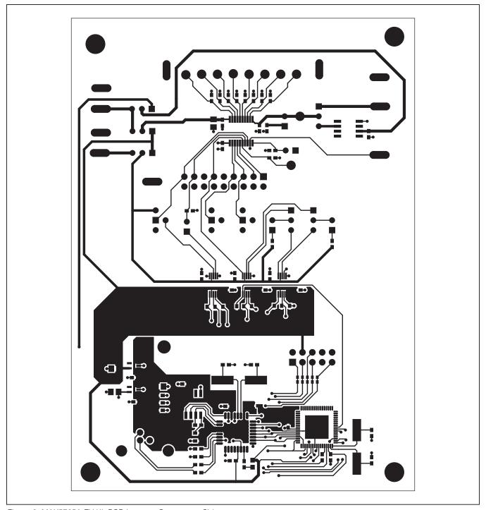
Figure 9. MAX5725A EV Kit PCB Layout—Component Side
