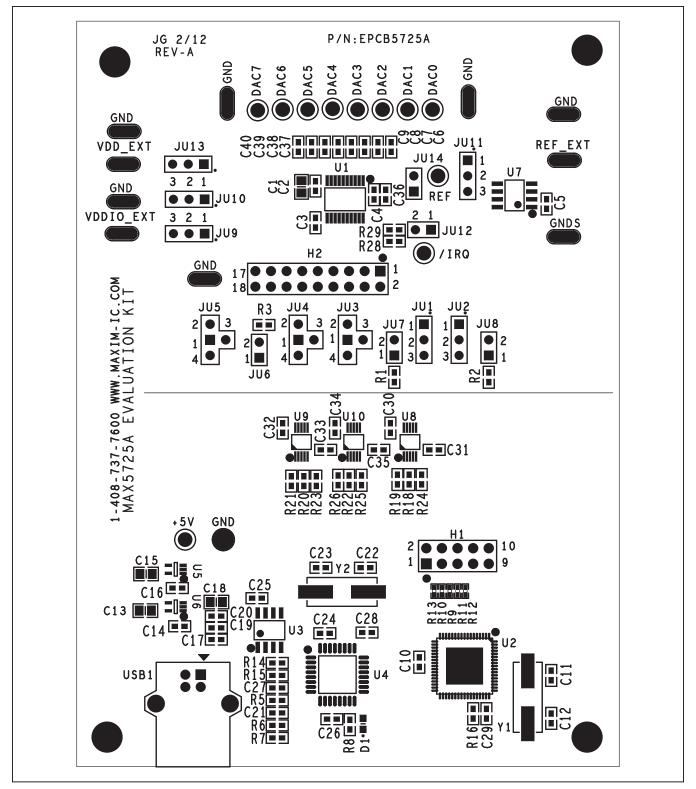
Figure 8. MAX5725A EV Kit Component Placement Guide—Component Side
