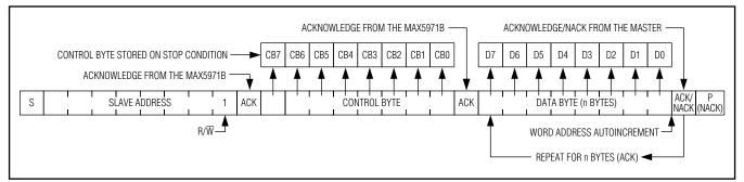
Figure 14. Read Format: Control and n Data Bytes Read
