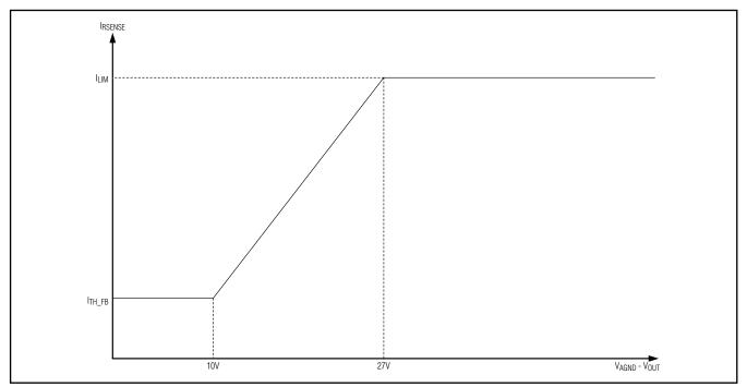
Figure 3. Foldback Current Characteristics
