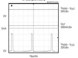
LED PWM TIMING: MAXIMUM DUTY **CYCLE (PROGRAMMABLE)**
