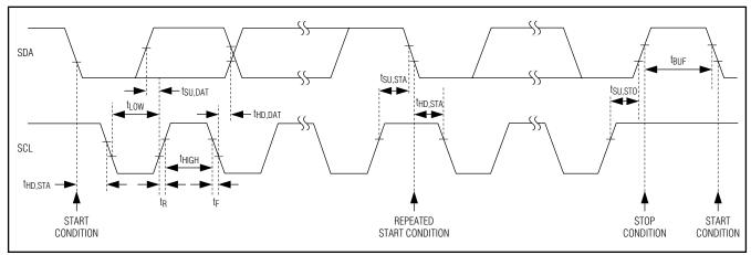
Figure 6. 2-Wire Serial Interface Timing Details
