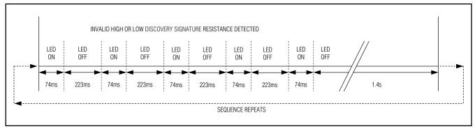
Figure 5. LED Code Timing for Detection Fault Due to High- or Low-Discovery Signature Resistance
