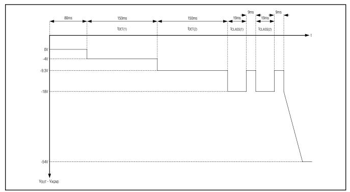
Figure 2. Detection, 2-Event Classification, and Port Power-Up Sequence
