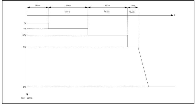
Figure 1. Detection, Classification, and Port Power-Up Sequence
