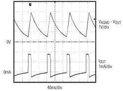
DETECTION WITH INVALID PD (33kQ) MAXS971B toc16c
