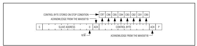
Figure 11. Write Format: Control Byte Received
