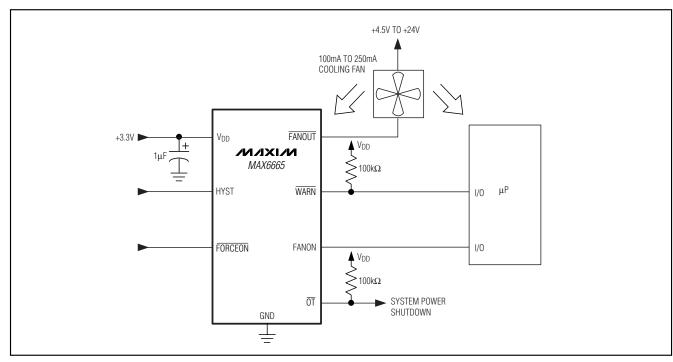
Figure 1. High-Reliability, Fail-Safe Fan Controller and Temperature Monitor
