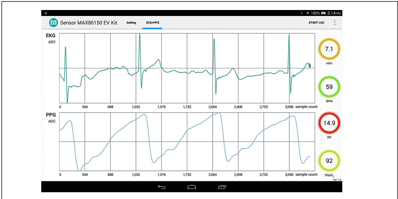
Figure 7. MAX86150 EV Kit ECG and PPG Waveform Display
