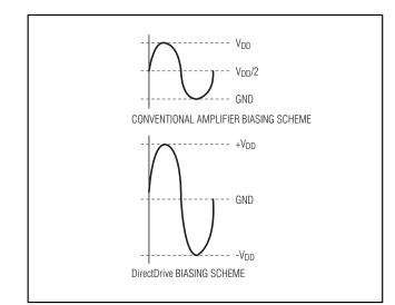
Figure 7. Traditional Amplifier Output vs. MAX9702 DirectDrive Output
