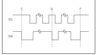
Figure 10. START, STOP, and REPEATED START Conditions
