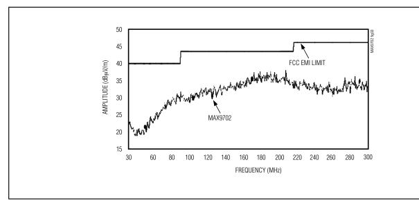
Figure 3. MAX9702 EMI with 76mm of Speaker Cable
