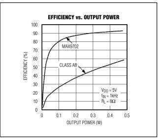
Figure 6. MAX9702 Efficiency vs. Class AB Efficiency
