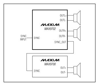
Figure 4. Cascading Two Amplifiers
