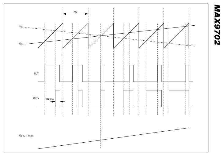
Figure 1. MAX9702 Outputs with an Input Signal Applied
