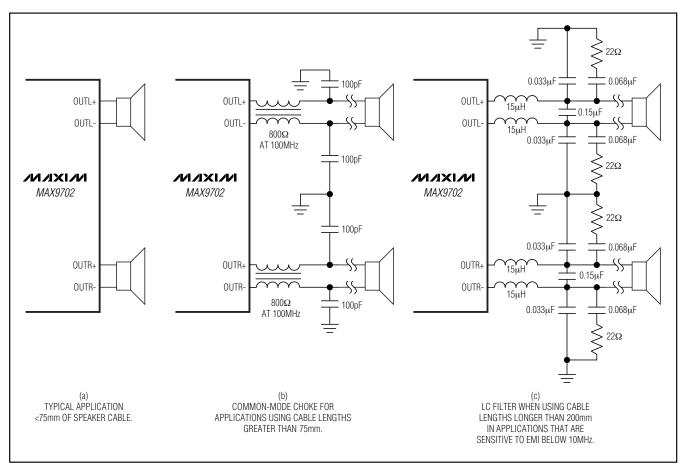
Figure 13. Optional Speaker Amplifier Output Filter
