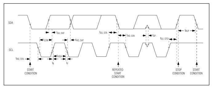
Figure 9. 2-Wire Serial-Interface Timing Diagram
