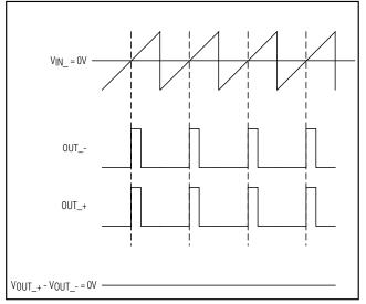
Figure 5. MAX9702 Outputs with No Input Signal
