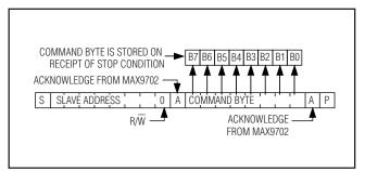
Figure 12. Write Data Format Example
