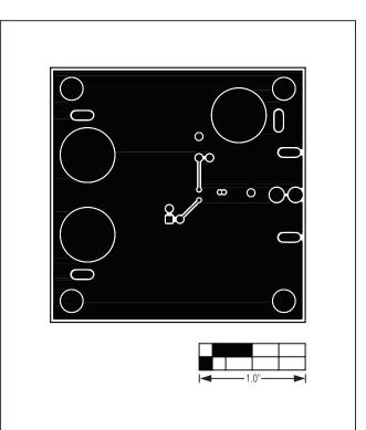
Figure 6. MAX98309 EV Kit PCB Layout—Solder Side
