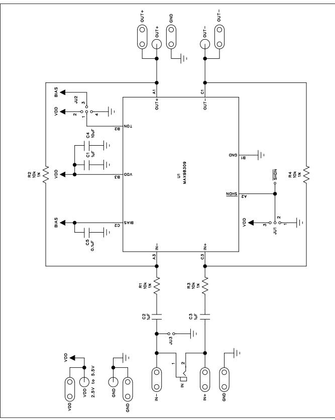
Figure 1. MAX98309 EV Kit Schematic
