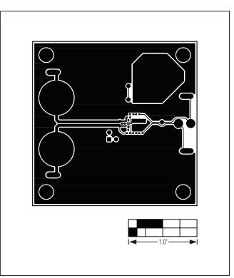
Figure 3. MAX98309 EV Kit PCB Layout—Component Side
