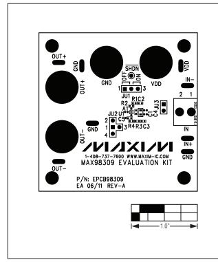
Figure 2. MAX98309 EV Kit Component Placement Guide— Component Side
