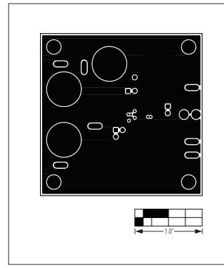
Figure 5. MAX98309 EV Kit PCB Layout—VDD Layer 3
