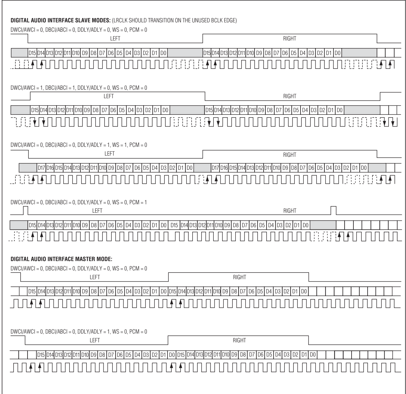
Figure 1. Digital Audio Interface Data Format Examples
