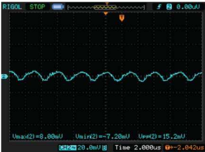
Figure 3. Output ripple at 2A load.
