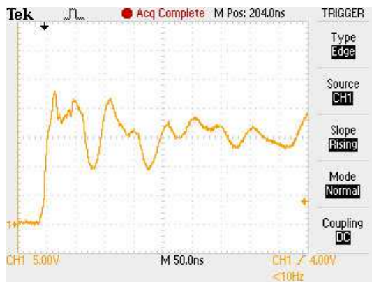
Figure 11. A 50ns time base oscilloscope shot of the 24V supply being hot-plugged into the Santa Cruz (M12-1).
