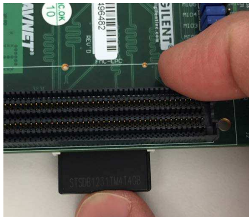
Figure 3. Inserting the SD card into the ZedBoard.
