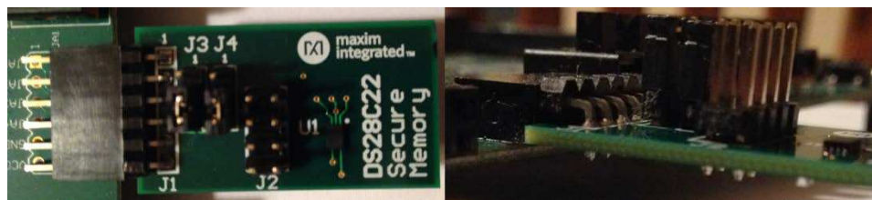
Figure 2. Pmod™ connector alignment.
