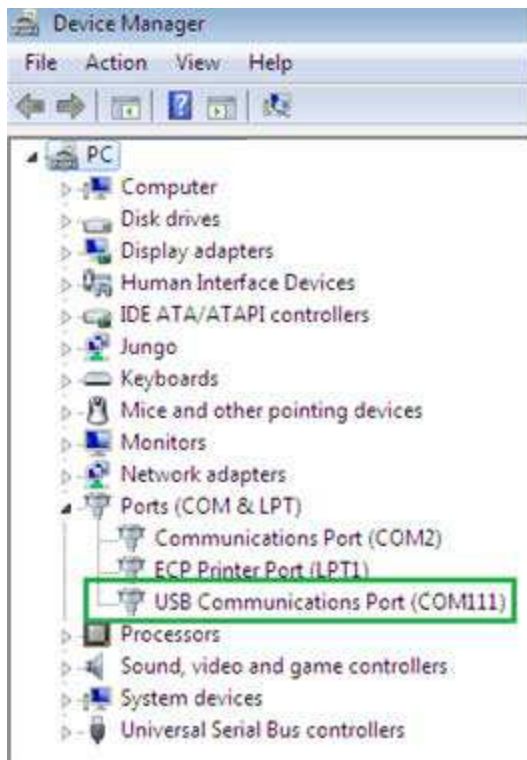
Figure 2. COM for for USB communication to the MAXREFDES46# board thru the USB type B connector at J6.
