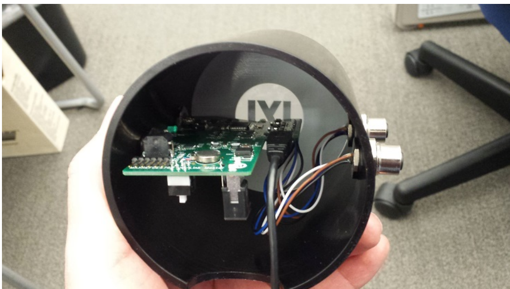
Figure 4. Connect the Micro-USB cable from underneath the MAXREFDES79# and then connect it to the PC.
