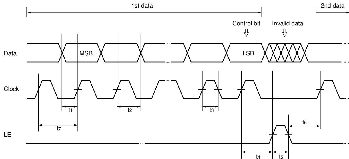
On the rising edge of the clock, one bit of data is transferred into the shift register.
