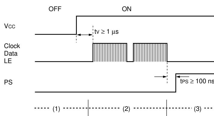
(1) PS = L (power saving mode) at Power ON
