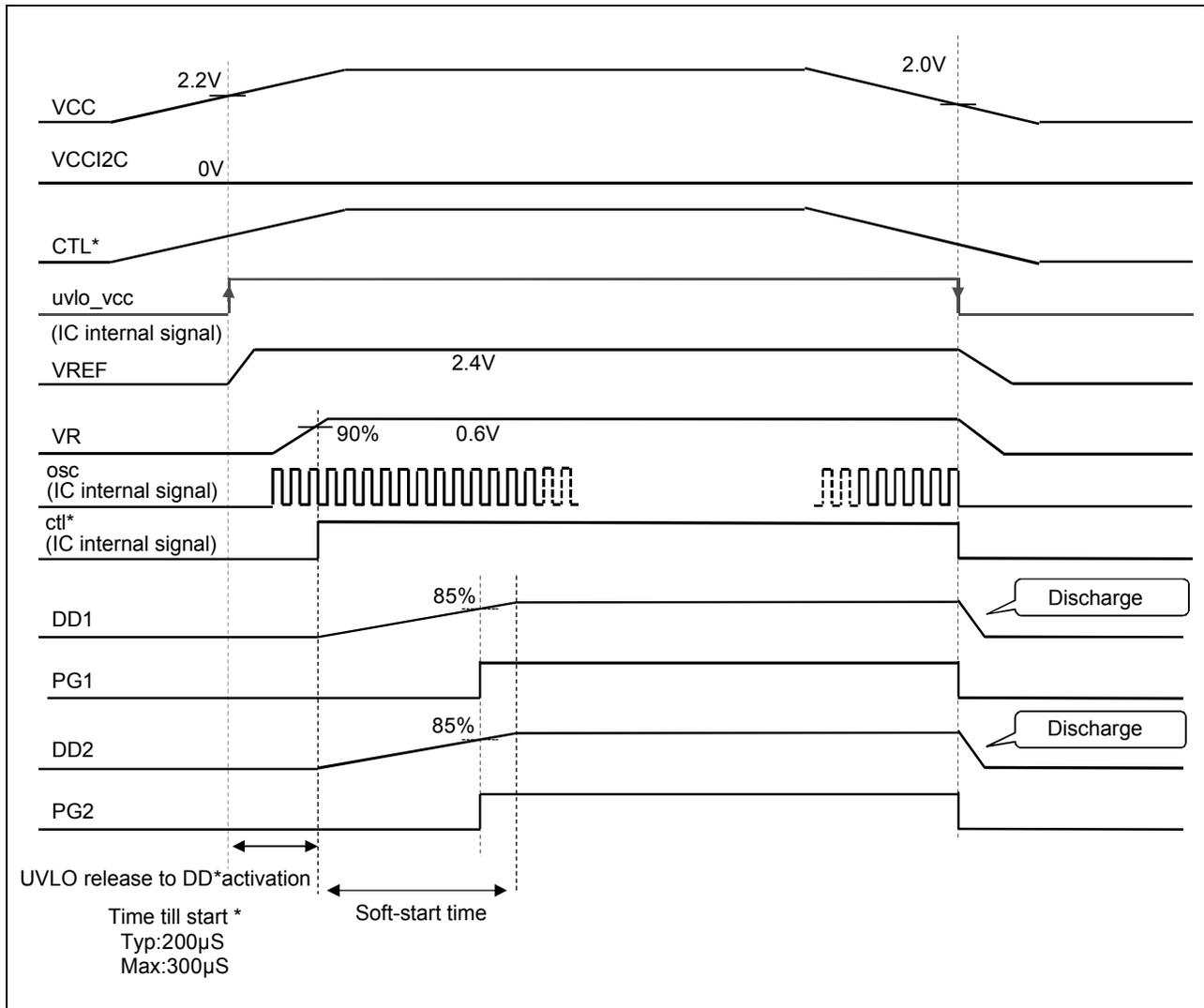
\*:VREF and VR activations depend on the VREF pin capacitance and VR pin capacitance. Time in the sequence figure above is applied for the following condition.
