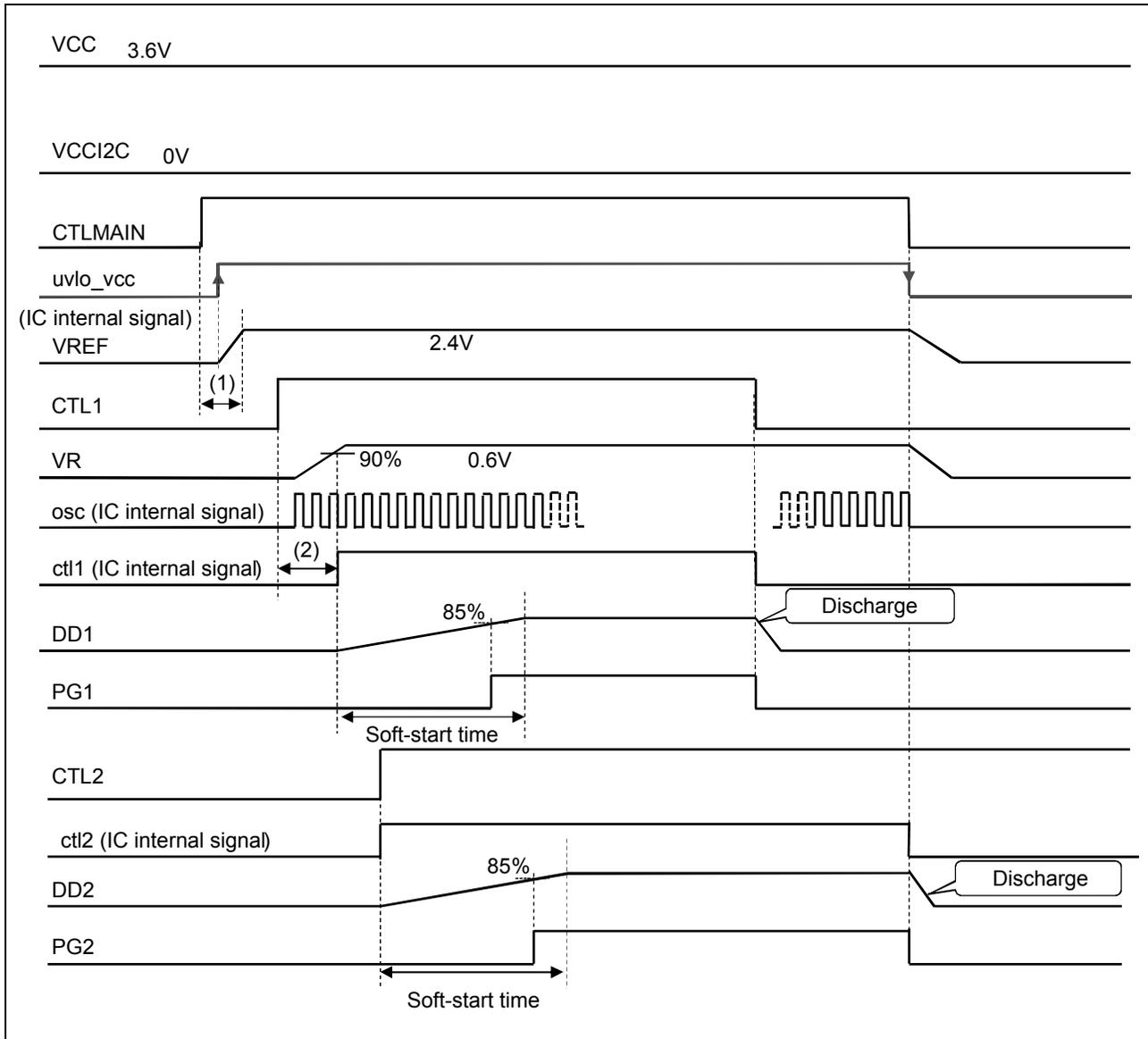
(1) Time from turning on CTLMAIN to VREF activation completion (=communication enabled)\*
