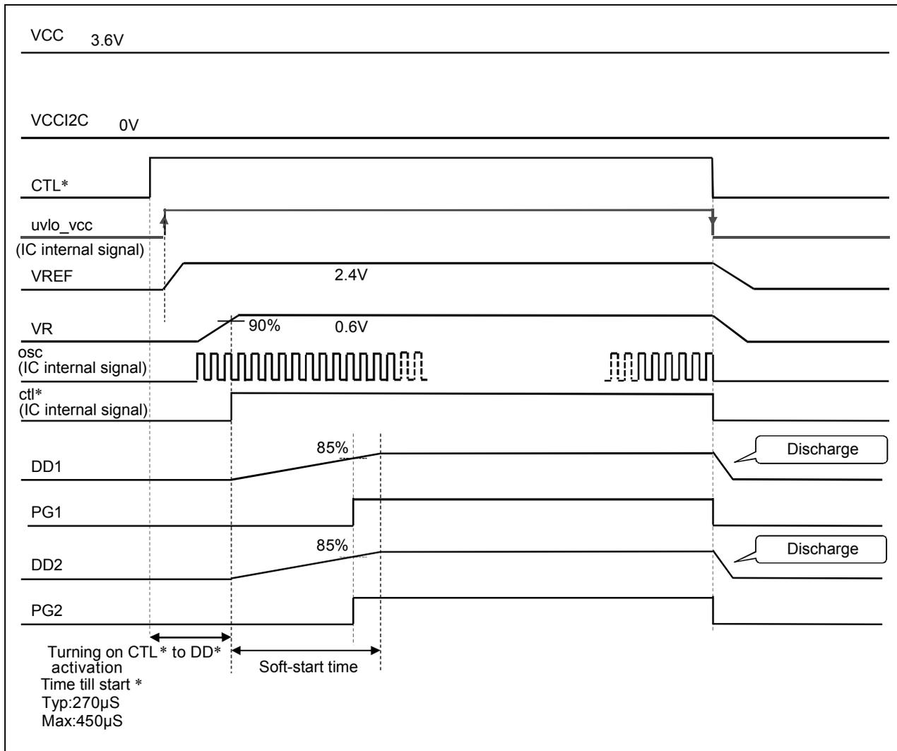
\*:VREF and VR activations depend on the VREF pin capacitance and VR pin capacitance.
