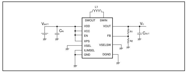
2. Using a selectable voltage option When VSEL = L  $\ensuremath{\mathsf{VSEL}}$
