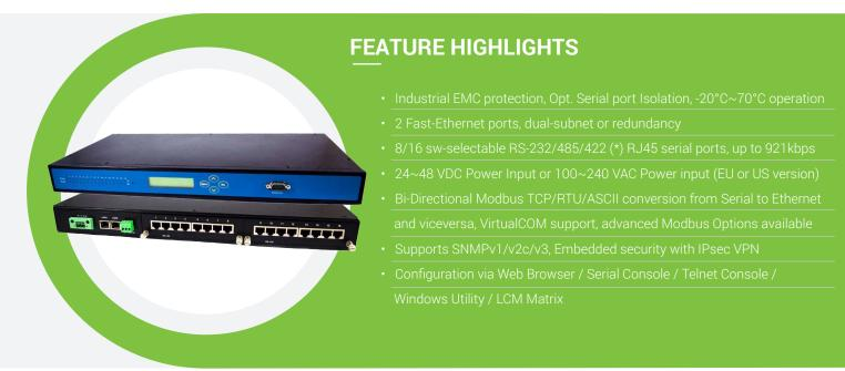
\*: RS-232/RS-485-RS-422 function is available on non-isolated versions. Isolated versions support RS-485 and RS-422 only
