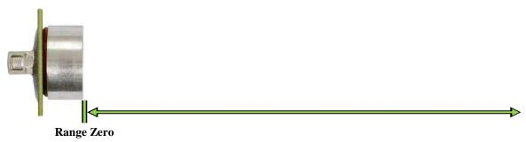
The range is measured from the front of the transducer to the target.
