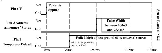
After the sensor is commanded to take a range reading it sends an ultrasonic pulse, waits between ~15ms to ~70ms to detect a target, and determines the range Then the sensor will resume I2C communications. If the sensor is addressed while in the middle of a range reading, all requests for communication will be responded with a NACK (not acknowledge).
