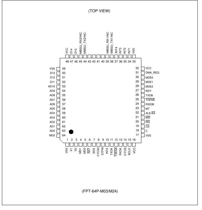
2. Pin assignment in 16 bit non-multiplexed parallel mode
