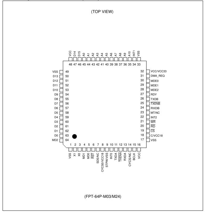
3. Pin assignment in SPI mode (MB88121B/C only)
