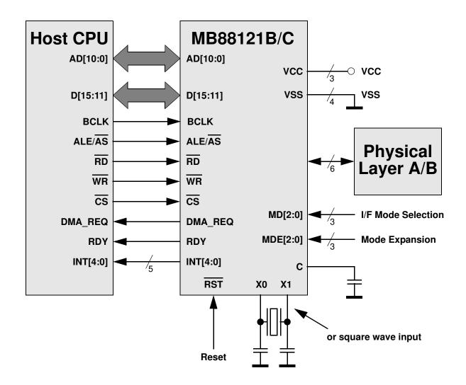
\*1: DMA\_REQ can only be used if RDY is not used, e.g. with automatic wait states. The initial function of the RDY/DMA\_REQ pin is RDY.
