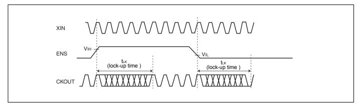
For modulation enable control using the ENS pin during normal operation, the set clock signal is output from CKOUT pin at most the lock-up time ( $t_{LK}$ ) after the level at the ENS pin is determined.
