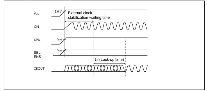
If the XPD pin is fixed at the "H" level, the maximum time after the power is turned on until the set clock signal is output from CKOUT pin is (the stabilization wait time of input clock to XIN pin) + (the lock-up time "tLK"). For the input clock stabilization time, check the characteristics of the resonator or oscillator used.
