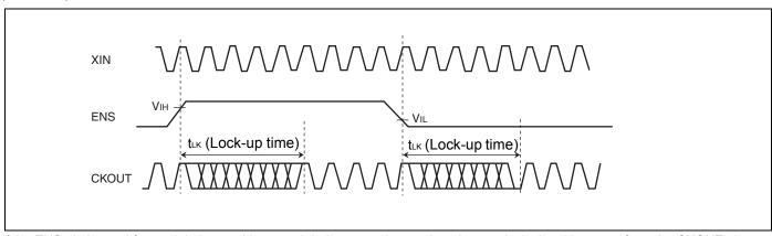
If the ENS pin is used for modulation enable control during normal operation, the set clock signal is output from the CKOUT pin at most the lock-up time "tuk" after the level at the ENS pin is determined.
