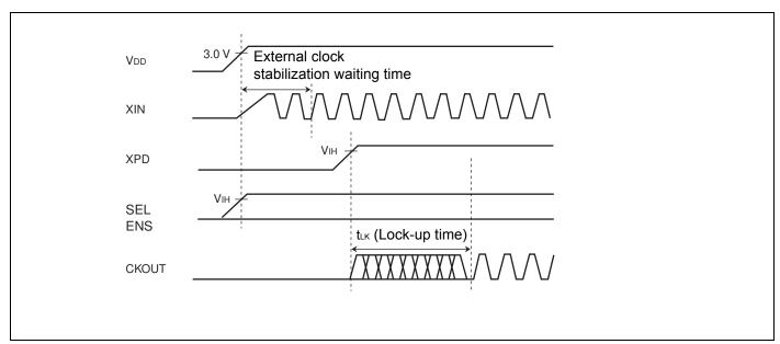
If the XPD pin is used for power-down control, the set clock signal is output from the CKOUT pin at most the lock-up time " $t_{LK}$ " after the XPD pin goes "H" level.
