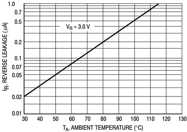
Figure 1. Reverse Leakage
