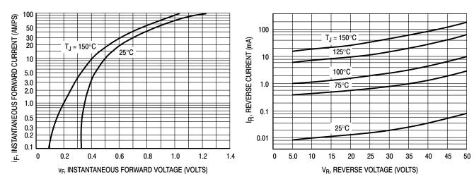
Figure 1. Typical Forward Voltage
