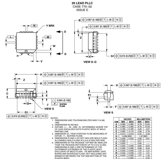
PLASTIC BODY. 7. DIMENSION H DOES NOT INCLUDE DAMBAR DIMENSION H DOES NOT INCLUDE DAMBAR PROTRUSION OR INTRUSION. THE DAMBAR PROTRUSION(S) SHALL NOT CAUSE THE H DIMENSION TO BE GREATER THAN 0.037 (0.940). THE DAMBAR INTRUSION(S) SHALL NOT CAUSE THE H DIMENSION TO BE SMALLER THAN 0.025 (0.635).
