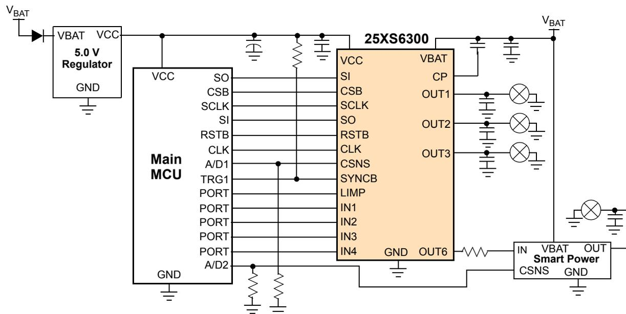
Figure 1. Triple 25 mΩ simplified application diagram
