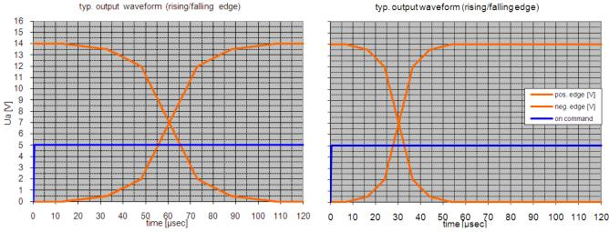
Figure 10. Typical power output switching (slow and fast slew rate)
