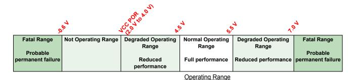
Figure 5. Ratings vs. operating requirements (VCC pin)
