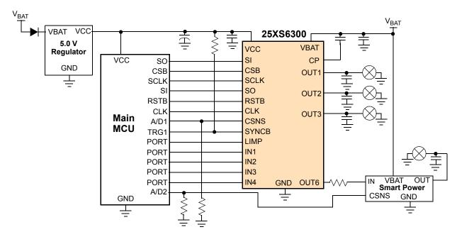
Figure 1. Triple 25 m $\Omega$  simplified application diagram
