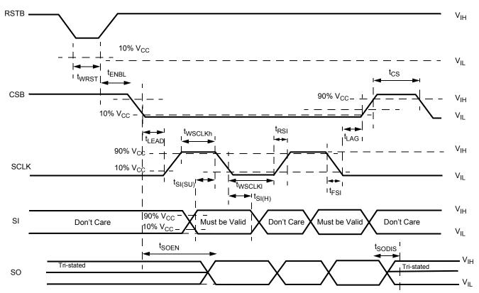
Figure 8. Timing requirements during SPI communication
