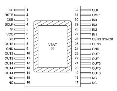
Figure 3. 12XS6 pinout diagram
