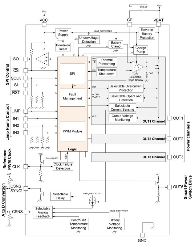
Figure 2. Simplified internal block diagram
