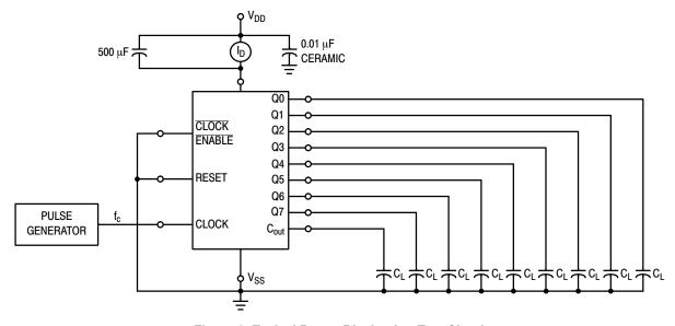
**Figure 2. Typical Power Dissipation Test Circuit**
