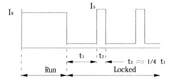
3rd wire signal Run : Square Wave Locked : Vaor V
