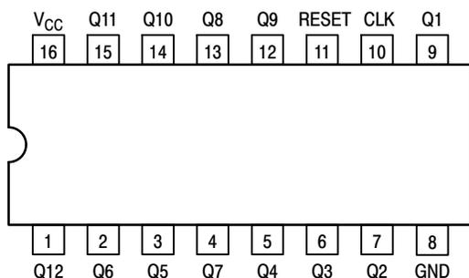
Figure 1. Pinout: 16-Lead Packages Conductors (Top View)
