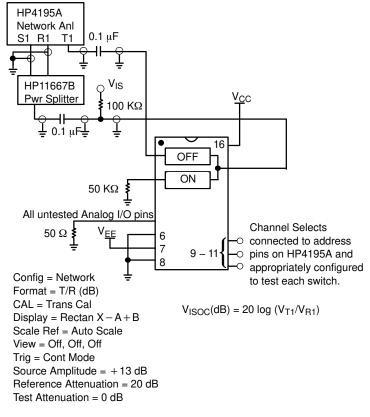
Figure 8. Maximum Common-Channel Feedthrough Isolation, Test Set-Up
