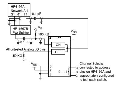
Figure 6. Maximum On Channel Bandwidth, Test Set-Up
