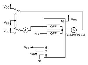
Figure 4. Maximum Off Channel Leakage Current, Any One Channel, Test Set-Up
