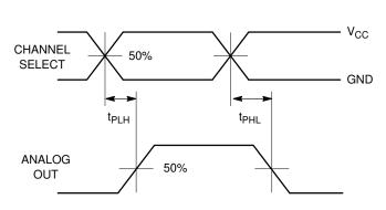
Figure 13. Propagation Delays, Channel Select to Analog Out
