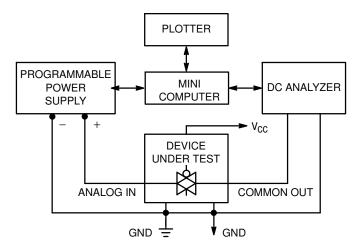
Figure 3. On Resistance, Test Set-Up
