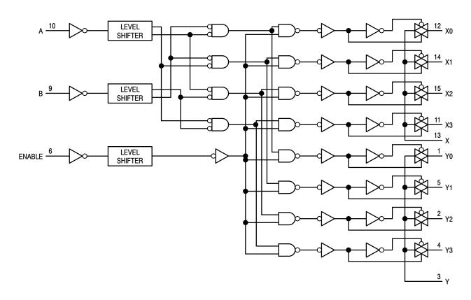
Figure 22. Function Diagram, LVX4052
