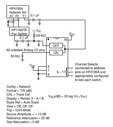
Figure 7. Maximum Off Channel Feedthrough Isolation, Test Set-Up
