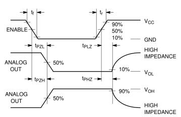
Figure 15. Propagation Delays, Enable to Analog Out
