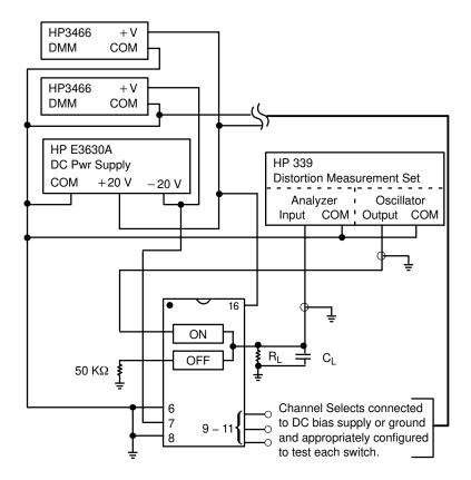
Figure 18. Total Harmonic Distortion, Test Set-Up
