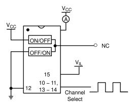
Figure 17. Power Dissipation Capacitance, Test Set-Up
