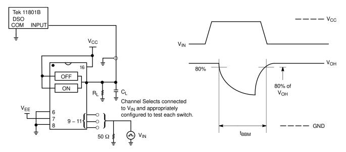
Figure 11. Break-Before-Make, Test Set-Up
