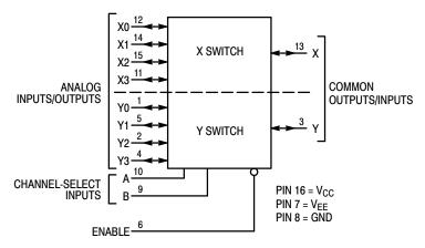
NOTE: This device allows independent control of each switch. Channel–Select Input A controls the X–Switch, Input B controls the Y–Switch.
