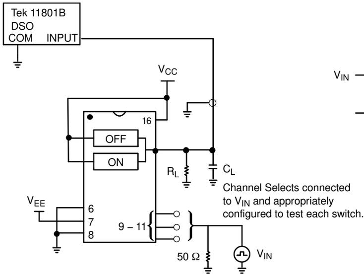
Figure 11. Break-Before-Make, Test Set-Up
