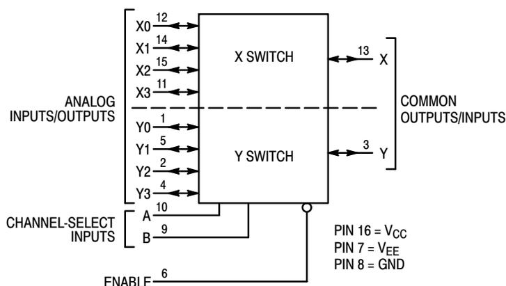
NOTE: This device allows independent control of each switch.
