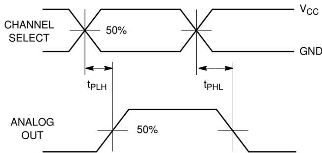
Figure 13. Propagation Delays, Channel Select to Analog Out
