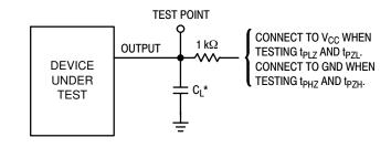
\*Includes all probe and jig capacitance
