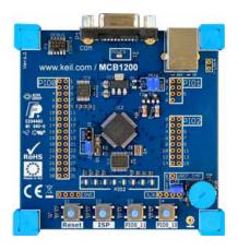
The Keil MCB1200 Evaluation Board enables you to create and test working programs based on the NXP LPC1200 family of ARM Cortex™-M0 processor-based devices.
